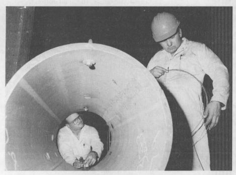
IN PREPARATION for cargo hold tests, Jeff Bobbe (left) and Mike Arviso (both 6642) install thermocouples on Sandia's simulated nuclear material transport cask, a five-ft-long, two-ft-diameter steel pipe. (Photo by Diana Helgesen, 2732)
